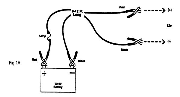
Connect one end of the red alligator clip to the positive terminal of a fully charged spare battery. Then connect one end of the black alligator clip to the negative terminal. Then connect the red alligator clip to the 12 volt output terminal on the alternator. Finally, connect the black alligator clip to a good chassis ground away from the battery compartment.
